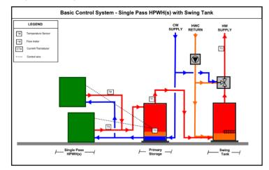
Figure 4. Swing Tank Configuration
